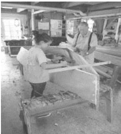
Checking to make sure the bottom will lie flat on the chines and transom.
